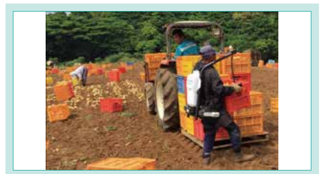
Fig. 2 Using a Power Assist Suit WIN-1 to Harvest Potatoes in a Field
