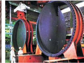
11 Valves used in water and sewerage lines to control the flow of fluids or gases.
