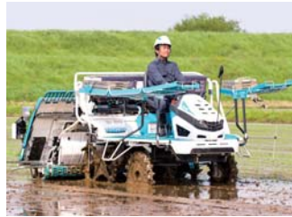
2 Rice transplanters: used to transplant rice seedlings to the rice paddies. Rice transplanters make a significant labor-saving contribution.
