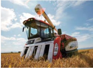
3 Combine harvesters: simultaneous harvesting and threshing of crops such as rice, wheat and pulses
