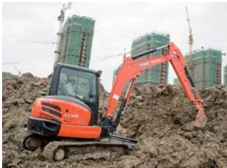
7 Construction machinery (mini backhoes): used in civil engineering and other operations; especially useful in narrow work areas, such as city streets.
