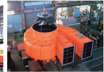
12 Pumps: used to pump water in water and sewerage lines, as well as in storm water drainage.
