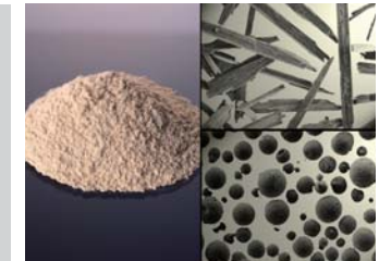
24 TXAX (brake pad material): used as a friction material, mainly in brake pads.
