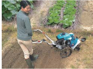
4 Mini power tillers: used mainly in agricultural operations, including smaller farms.
