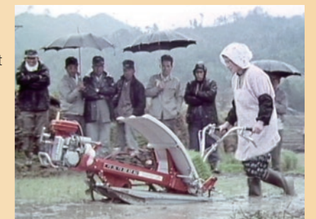
Full-automatic walk-behind rice transplanter (SPS type), the original model for subsequent transplanters
