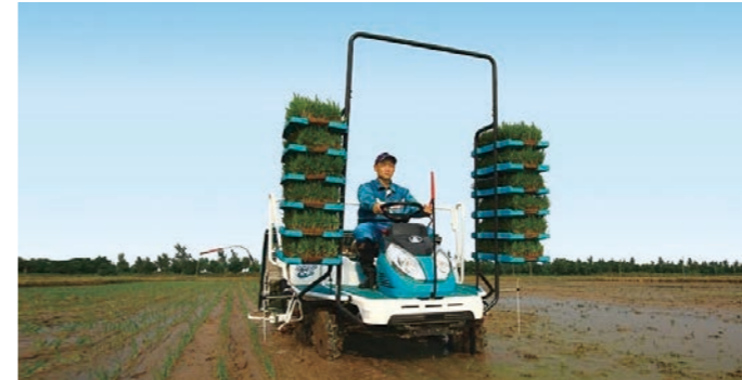
Rice transplanters: used to transplant rice seedlings to rice paddies, contributing significantly to labor saving.
