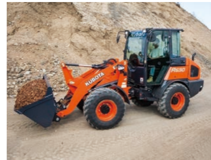
Wheel loaders: used mainly for transporting and stacking tasks (at construction sites, farms, etc.).
