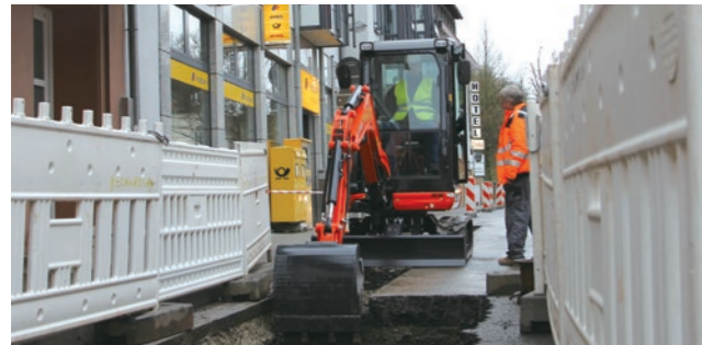
Mini excavators: used in civil engineering and other operations; especially useful in narrow work areas, such as city streets.
