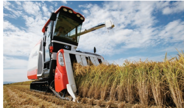
Combine harvesters: used for simultaneous harvesting and threshing of crops such as rice, wheat and pulses.
