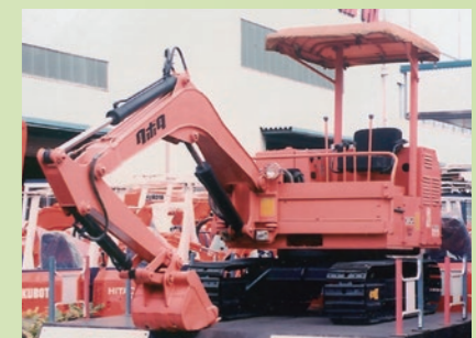
Full-revolving small hydraulic shovel (KH1), the base model for subsequent Kubota mini excavators
