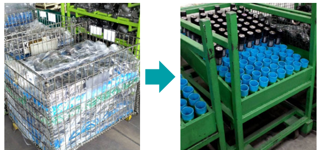
At Kubota Precision Machinery (Thailand) Co., Ltd., we revised plastic film packaging for components and changed to reusable racks, which has reduced plastic and labor.
