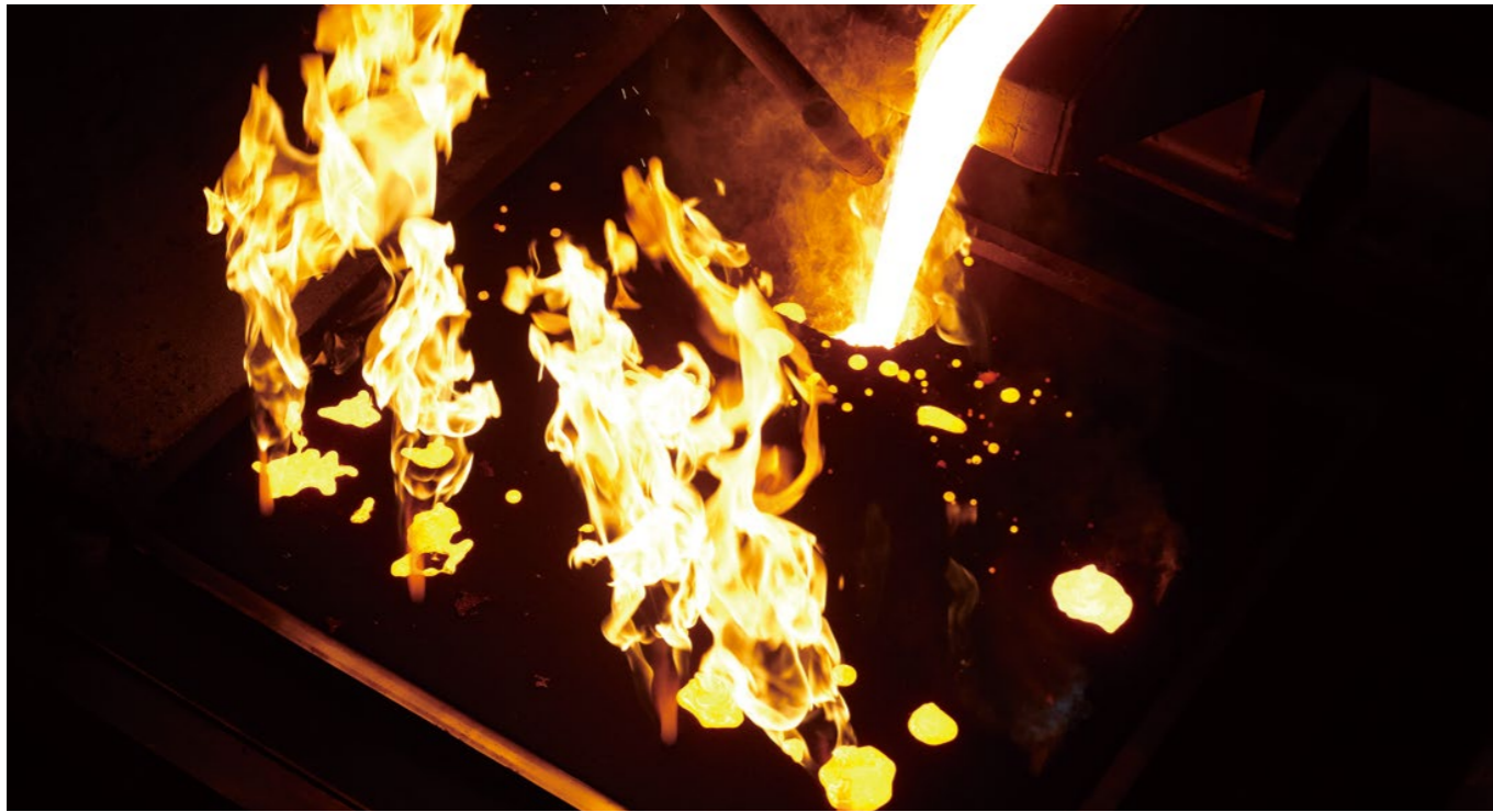
Manufacturing cast parts at SKMT involves pouring red-hot iron into a mold.
