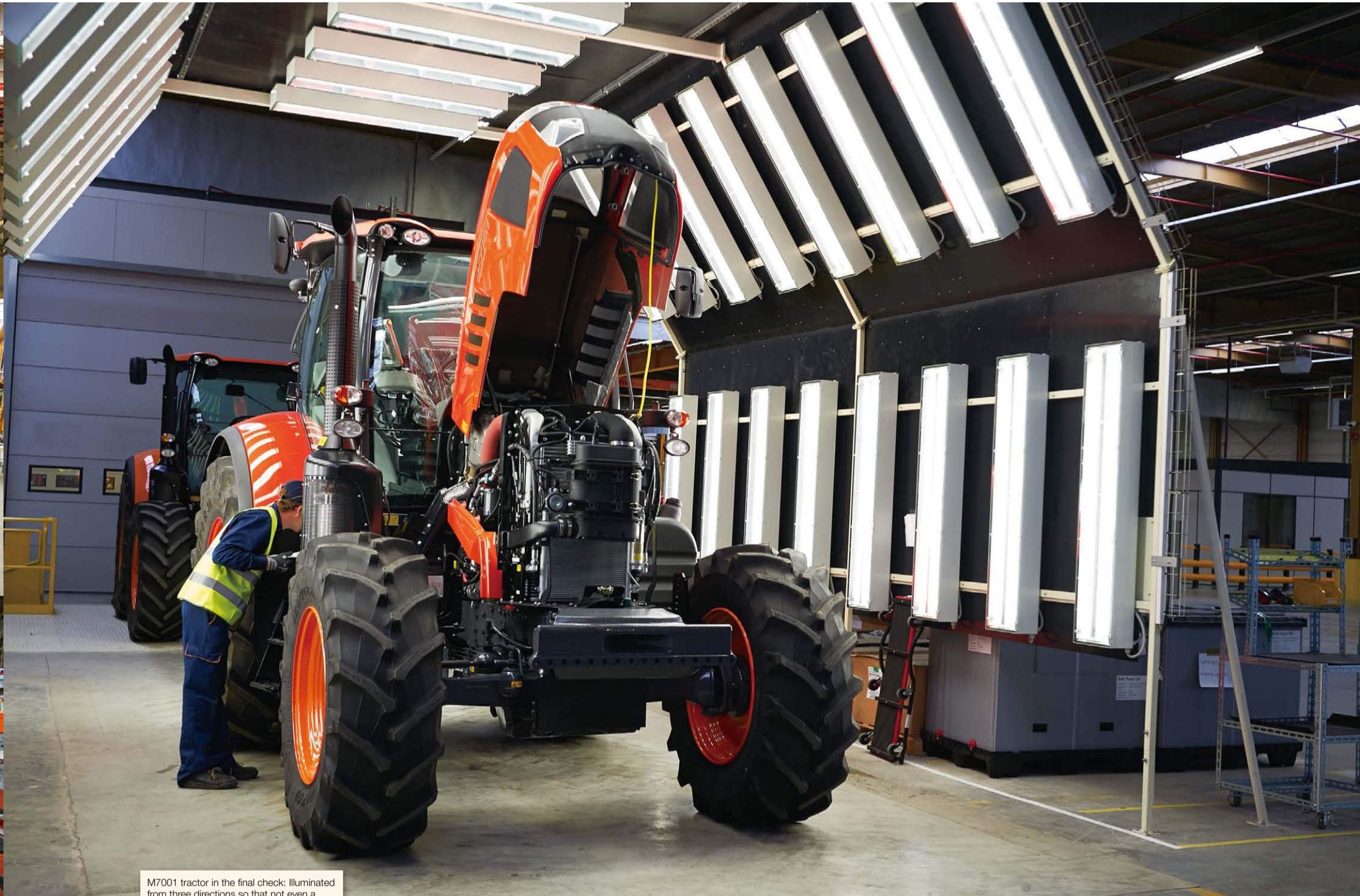
M7001 tractor in the final check: Illuminated from three directions so that not even a scratch will be overlooked.
