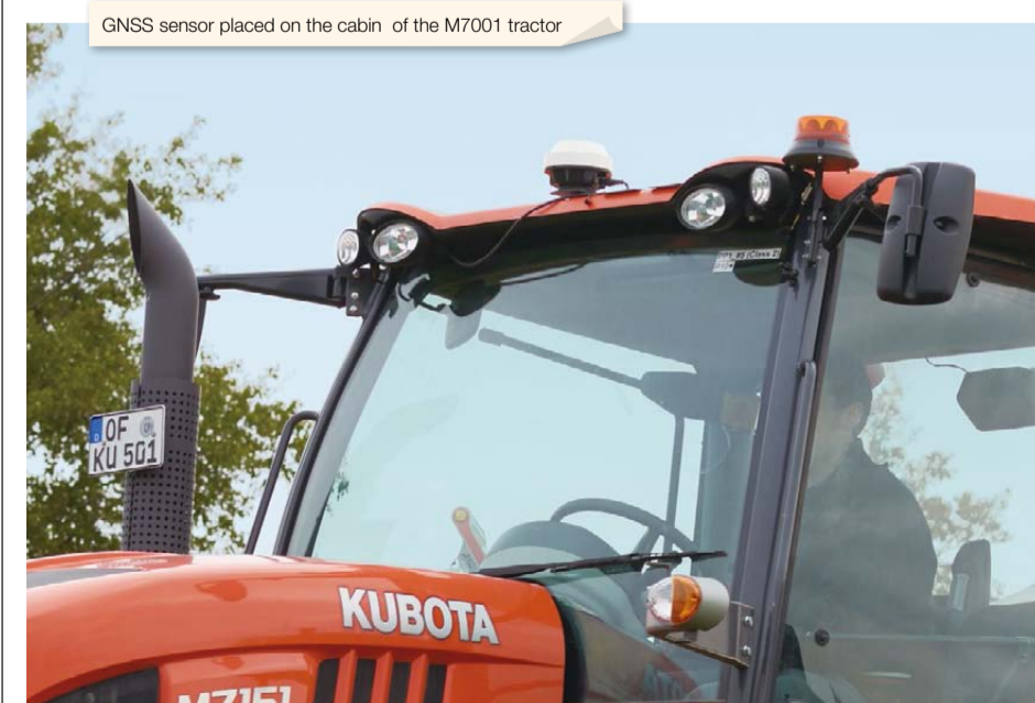
GNSS sensor placed on the cabin of the M7001 tractor
