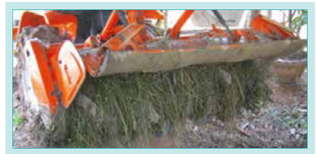
Fig. 9 Pulled-up Stalks Jamming into Rotary Machine
