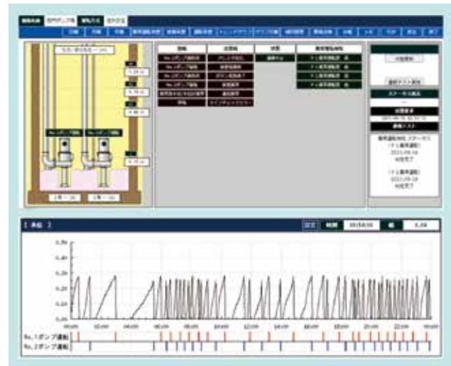
Fig. 3 Cloud Monitoring Screen Example
