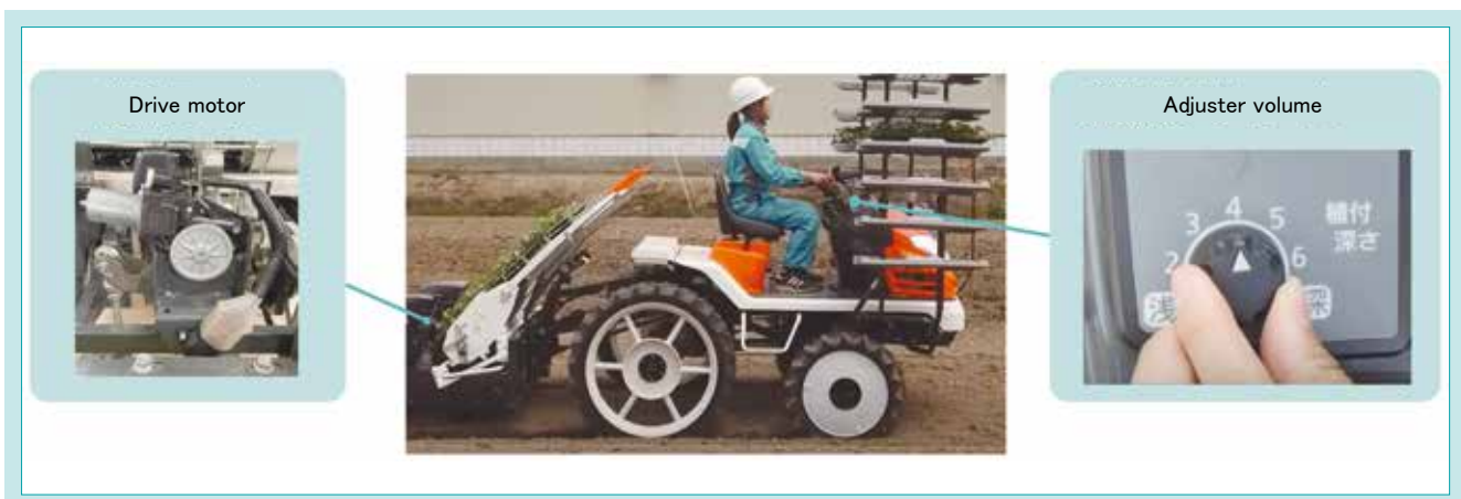
Fig. 13 Planting Depth Adjustment Structure
