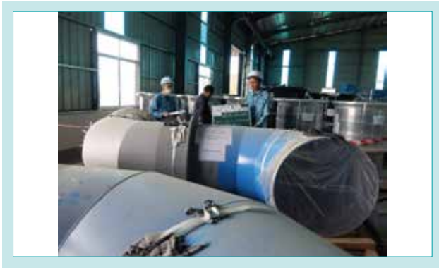
Fig. 5 Acceptance Inspection (Steel Pipe)
