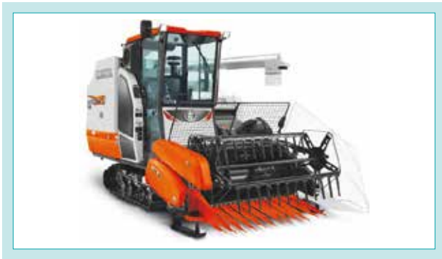
Fig. 2 Corn Kit CK70 Attached to DC70
