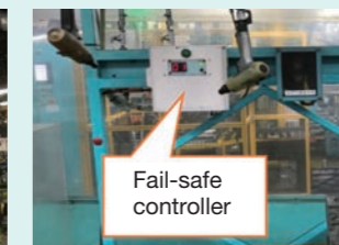
Fail-safe equipment prevents workers from forgetting to tighten bolts or applying insufficient torque. If a worker does forget, the equipment does not let them proceed to the next task.
