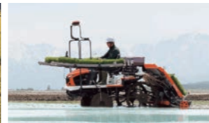
KSAS-compatible rice transplanter with an electric fertilizer volume control unit
