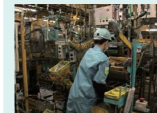
Components are provided from in front and tools are all within 40 cm of the worker, enabling them to get on with their work close at hand without twisting to look or walking around.
