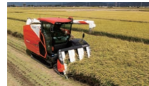
KSAS-compatible combine harvester with a taste and yield sensor
