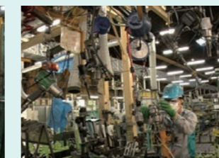
The system brings down the tools needed at the time they are needed. Four wasteful movements—crouching, walking, reaching, and searching—have been improved.
