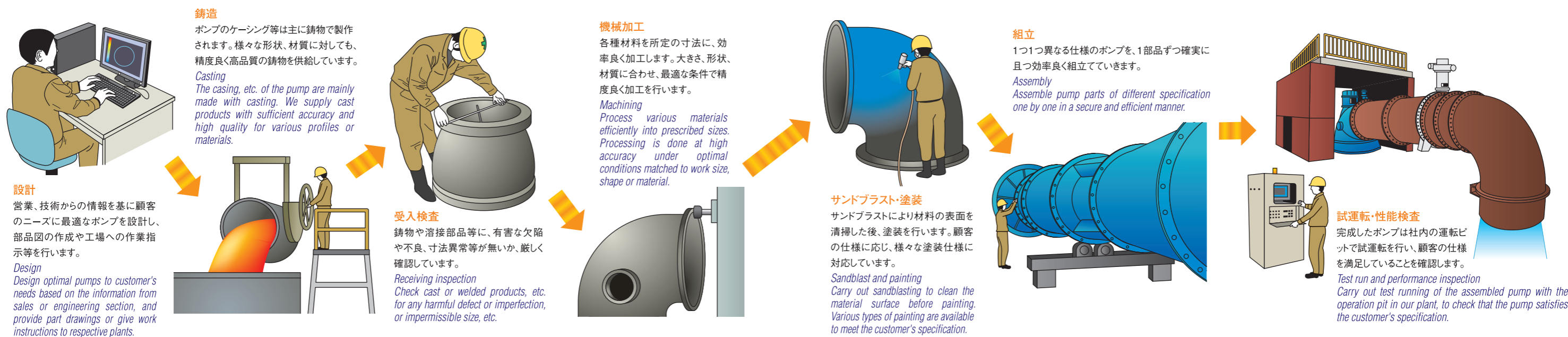
立軸斜流ポンプ (DF-V型) Vertical mixed flow pump (model: DF-V) 口径: 200~3400mm 吐出量: 4~1800m 3 /min 全揚程: 5~150m 用途: 上下水道、雨水排水、工業用水、農業用水、冷却水、消火用水、海水取水・送水等 Diameter: 200 - 3400 mm Discharge capacity: 4 - 1800 m 3 /min Total head: 5 - 150 m Use: Water and sewage, rain water drainage, industrial water, water for agricultural use, cooling water, fire-fighting water, seawater intake, water supply, etc.
