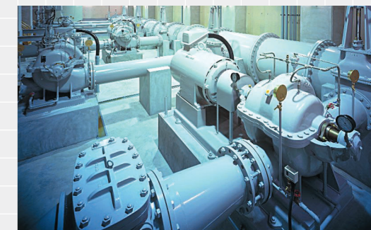
両吸込み渦巻ポンプ (DV-L型) Double suction centrifugal pump (model: DV-L) 口径: 200~1600mm 吐出量: 2.6~400m 3 /min 全揚程: 5~200m 用途: 上下水道、工業用水、農業用水、冷却水、消火用水等 Diameter: 200 - 1600 mm Discharge capacity: 2.6 - 400 m 3 /min Total head: 5 - 200 m Use: Water and sewage, industrial water, water for agricultural use, cooling water, fire-fighting water, etc.
