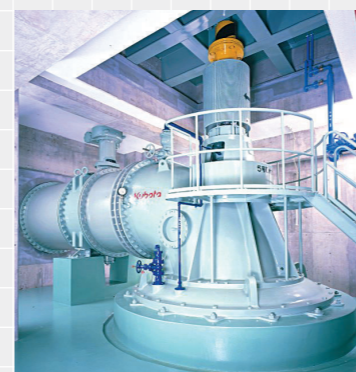
立軸斜流ポンプ (DF-V型) Vertical mixed flow pump (model: DF-V) 口径: 200~3400mm 吐出量: 4~1800m 3 /min 全揚程: 5~150m 用途: 上下水道、雨水排水、工業用水、農業用水、冷却水、消火用水、海水取水・送水等 Diameter: 200 - 3400 mm Discharge capacity: 4 - 1800 m 3 /min Total head: 5 - 150 m Use: Water and sewage, rain water drainage, industrial water, water for agricultural use, cooling water, fire-fighting water, seawater intake, water supply, etc.
