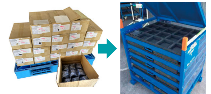
At Kubota Precision Machinery (Thailand) Co., Ltd., we reviewed our use of single-use cardboard and plastic film packaging in an effort to reduce waste and conserve labor resources.
