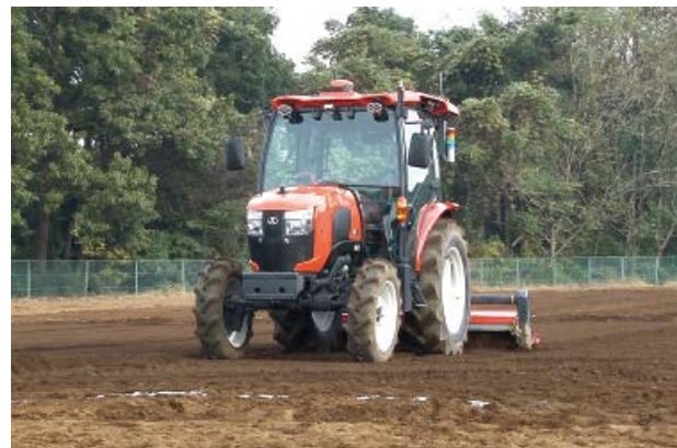
Autonomous tractor (under development)
