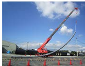
Earthquake-resistant ductile iron pipe GX-type DN(Nominal diameter) 400
