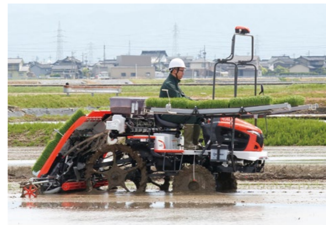
Rice transplanters: used to transplant rice seedlings to rice paddies, contributing significantly to labor saving.
