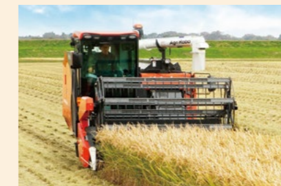
AGRIROBO Combine harvester with automated driving assist function
