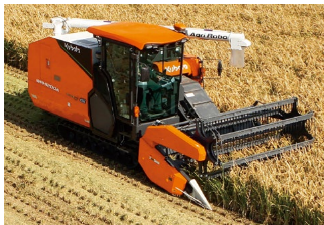
Combine harvesters: used for simultaneous harvesting and threshing of crops such as rice, wheat and pulses.
