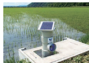
The WATARAS field water management system
