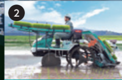
2 Rice transplanters: used to transplant rice seedlings to the rice paddies. Rice transplanters make a significant labor-saving contribution.
