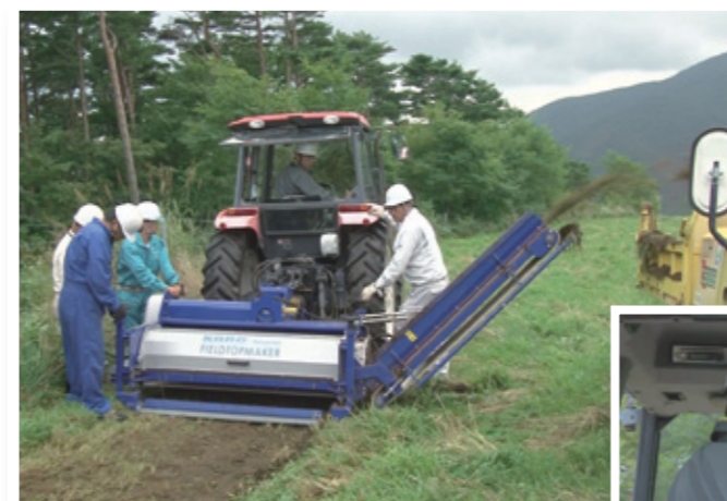
Decontamination with tractor attached implement
