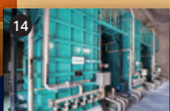
14 Ceramic film: used in the purification process for sources of water, including river water, to create clean drinking water.
