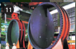
11 Valves: used in water and sewerage lines to control the flow of fluids or gases.
