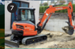
7 Construction machinery (mini backhoes): used in civil engineering and other operations; especially useful in narrow work areas, such as city streets.
