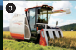
3 Combine harvesters: simultaneous harvesting and threshing of crops such as rice, wheat and pulses
