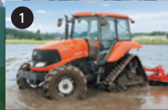
1 Tractors: used mainly in agricultural operations, including tillage, leveling and transportation.
