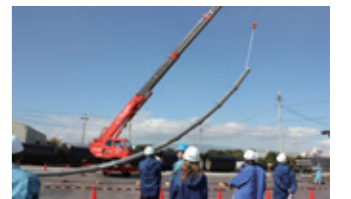
Testing a pipe for earthquake resistance
