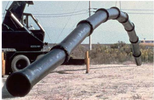
Hoisting test for a ductile iron pipe using earthquake-resistant joints
