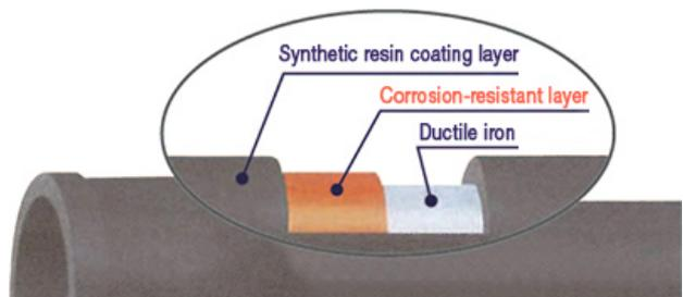
External corrosion-resistant coating C-Protect (conceptual image)
