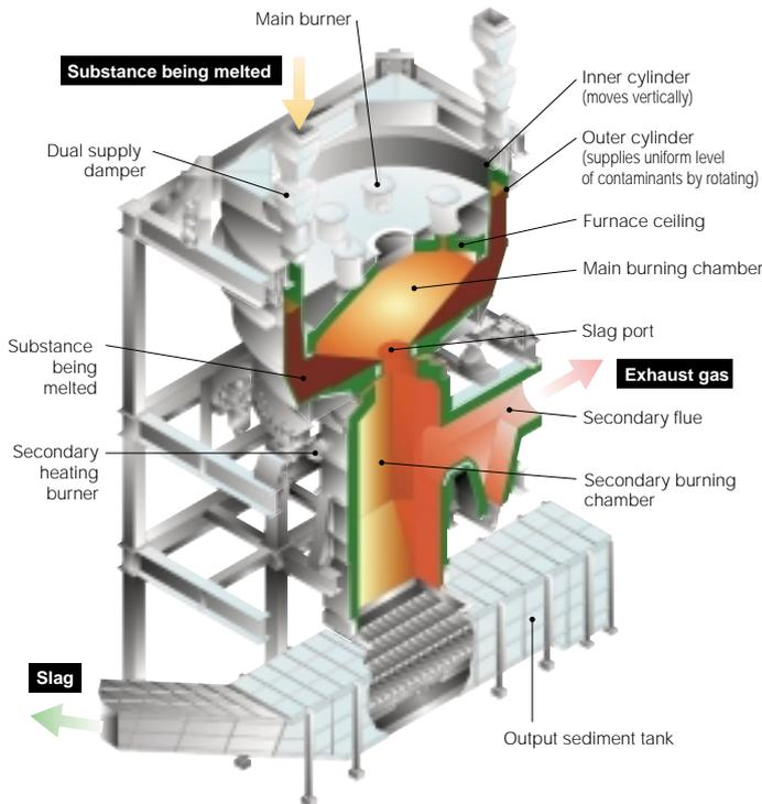
Structure and operation of the melting furnace
