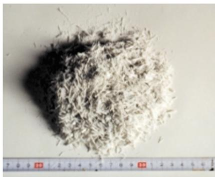
Photo 2. Recycled material from FW pipes (FRP layer)
