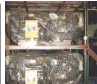
Effect: We reduced the amount of waste in our customers, and made unpacking easy, by changing crate from wood to steel. ( We reduced nine tons of carbon dioxide annually, and 5.49 million yen in cost annually. )
