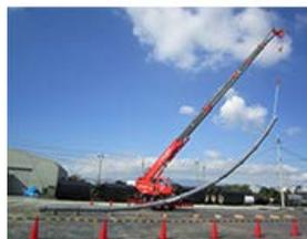
Earthquake-resistant ductile iron pipe
