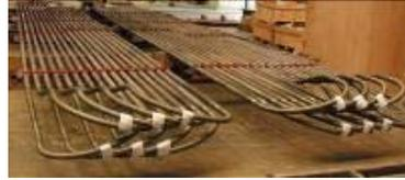
Cracking tubes for ethylene
