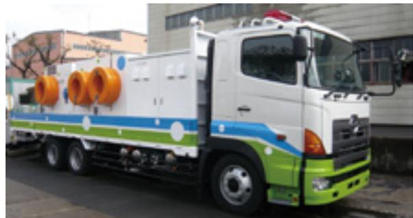
Drainage Pump with Vehicle for Disaster Recovery
