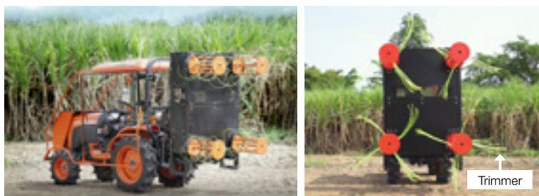
SLR110H mounted on a small tractor
