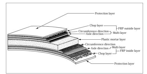
Figure 1. Structure of FW pipe
