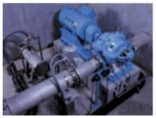
Pump with reverse rotation impeller
