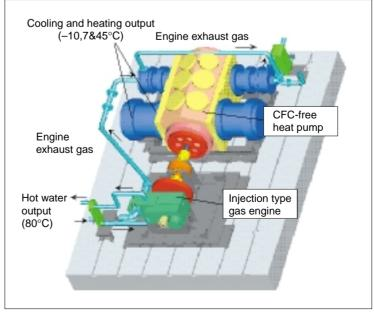
Schematic of system configuration
