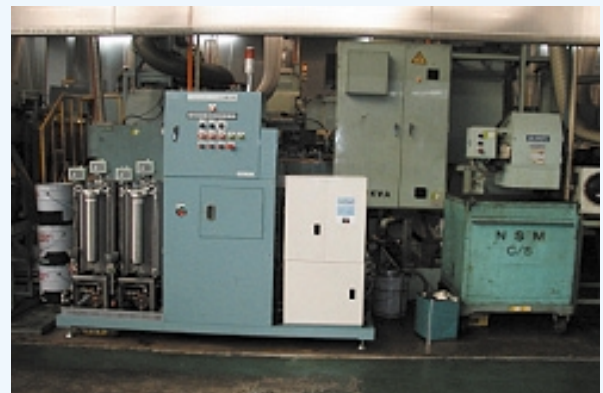
Alkaline ionizing equipment for cutting oil
