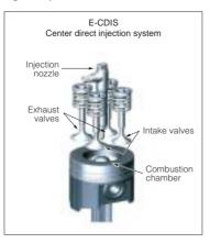
pressure injection and newly optimized combustion chamber. These engines are highly accepted by our customers inside and outside of our company as the engines which complied with the exhaust gas regulations all over the world with the performance of compact, high power, low noise and low vibration as well as high reliability.
