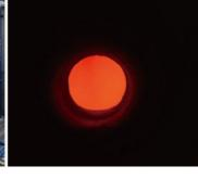
Interior of the incinerator as seen from the viewing window. By switching from ordinary incineration (800°C) to high-temperature incineration (850°C), the circulating fluidized bed incinerator can reduce N2O emissions by approximately 60%.
