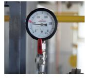
Pressure gauge for city gas supplied to the gun burner
