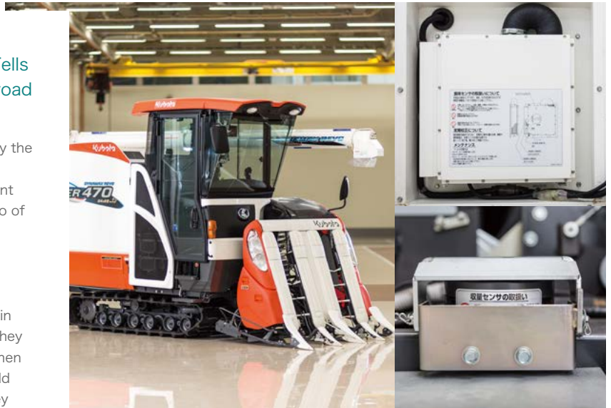
With the taste-yield sensor installed, data on crop quality can be collected at the time of harvesting
