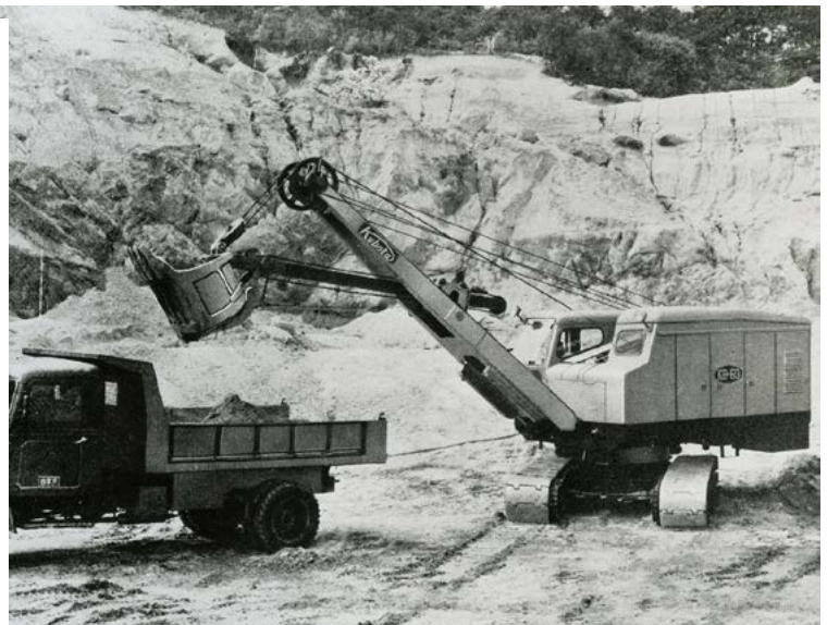
Non-hydraulic Excavator KB60 loading at a construction site
