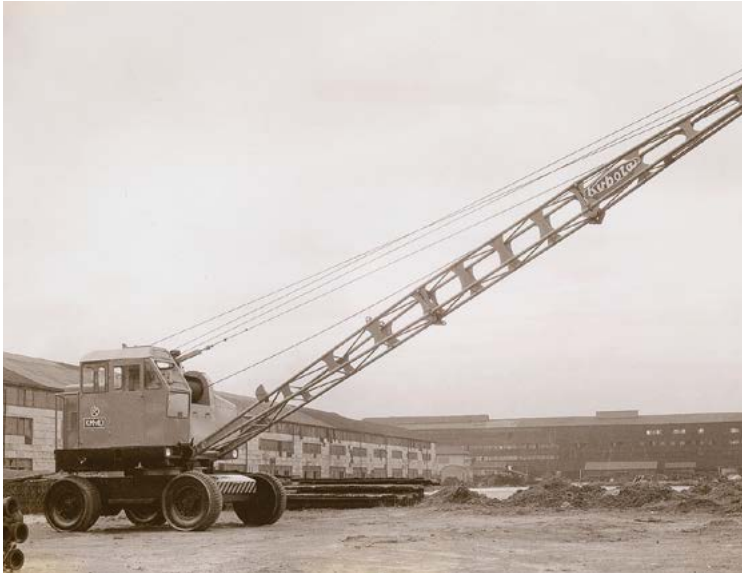
The KM40 Type Mobile Crane tested at the Mukogawa machinery plant
