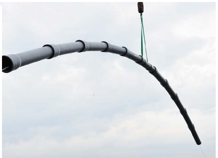
Pipeline suspension test for Kubota's earthquake-resistant ductile iron pipes. The joint section flex considerably, preventing detachment
