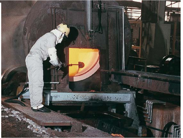
Centrifugal casting of ductile iron pipes using resin sand
