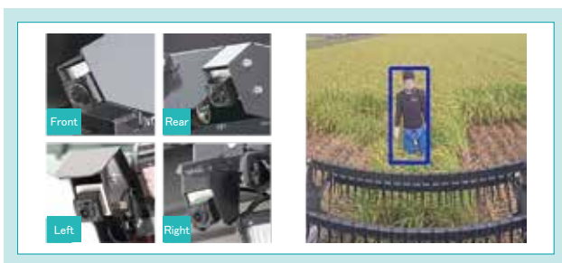
Fig. 6 Camera Mounted Around the Combine Harvester and Person Detection
