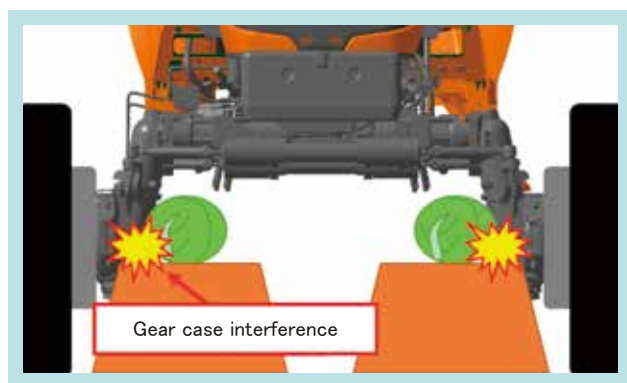
Fig. 6 Interference Between the Gear Case and the Crop
