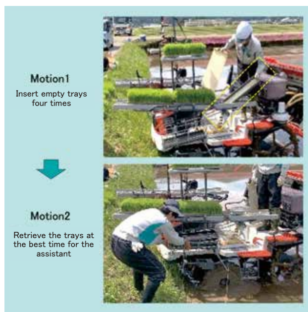
Fig. 12 Operational Actions Using the New Mechanism
