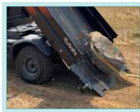
Fig. 12 Cargo Extended Gate
