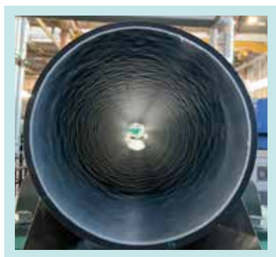
Fig. 7 Inner Surface of HTPP Before the Improvement of Unevenness
