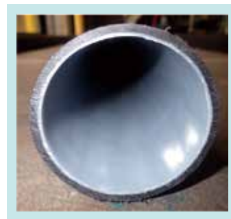
Fig. 6 Inner Surface of Improved Impact-Resistant HTPP
