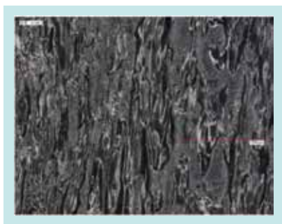
Fig. 3 Surface of Leaking HTPP
