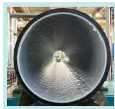
Fig. 8 Inner Surface of HTPP After the Improvement of Unevenness
