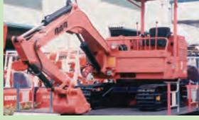
Fully revolving small hydraulic shovel, the base model for subsequent Kubota mini excavators
