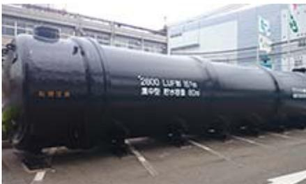
An earthquake-resistant water storage tank
