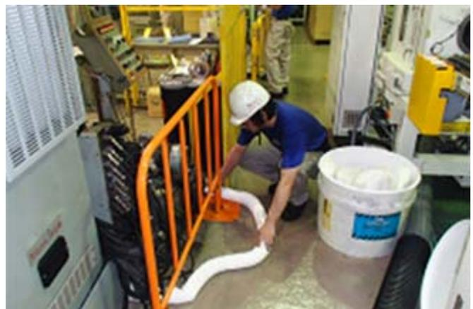
Flow prevention drill simulating the leakage of oil.
