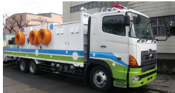
Drainage Pump with Vehicle for Disaster Recovery
