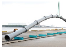
Installed earthquake-resistant ductile iron pipes for the first time in the U.S.
