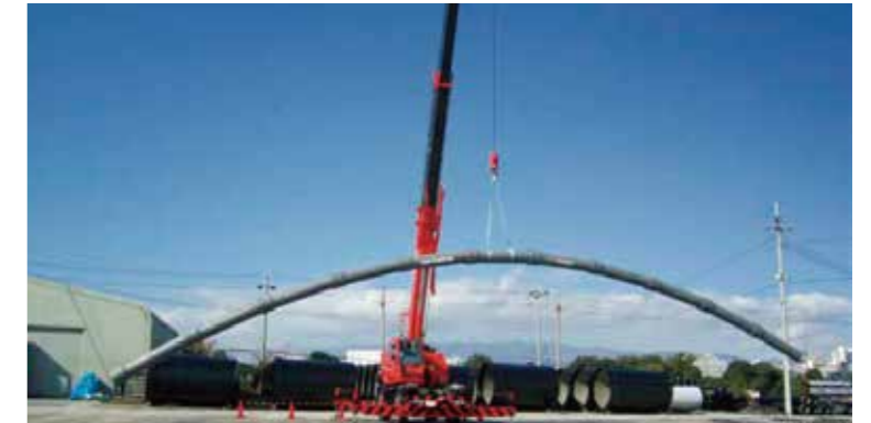
Hanging test of earthquake resistant joint
