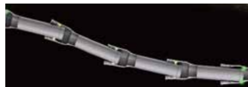
Chain Structure pipeline can adjust ground deformation with joint deflection performance.
