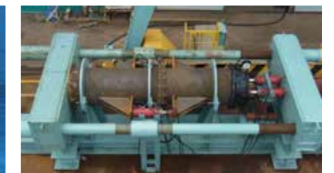
The pipes are tested by hydraulic pressure.
