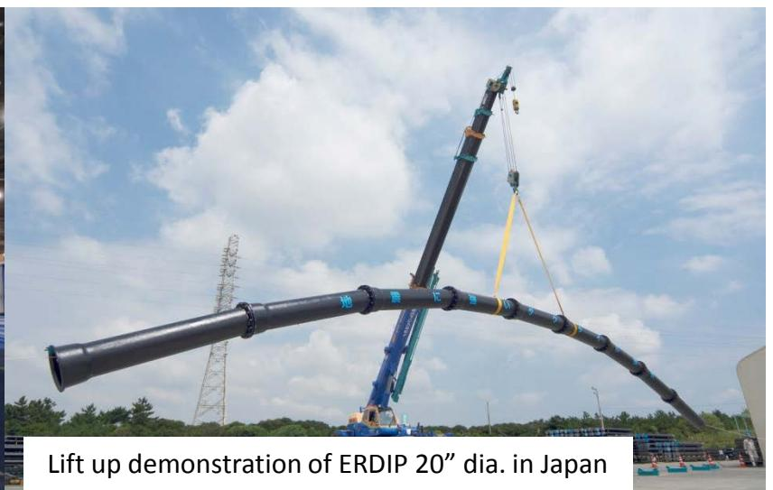
Lift up demonstration of ERDIP 20" dia. in Japan
