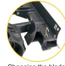
Changing the blade width is as easy as removing one pin by hand.
