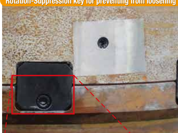
Rotation-Suppression key for preventing from loosening
