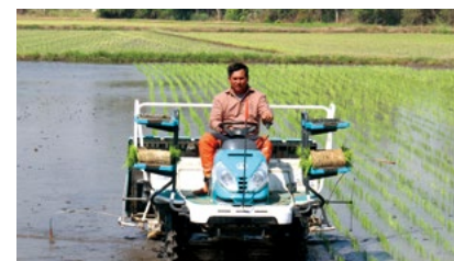
The use of rice transplanters boosts productivity substantially compared to traditional agriculture using human labor.
