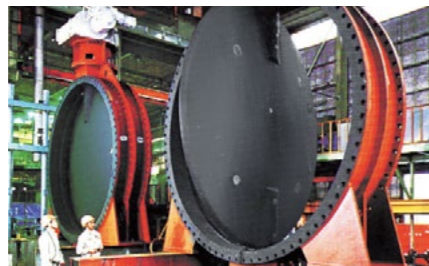
Valves: used to control the flow of fluids or gases in water and sewerage lines, agriculture and forestry, and the rainwater market.
