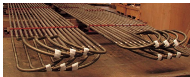
Cracking coil used at petrochemical plants for ethylene purification and other operations.
