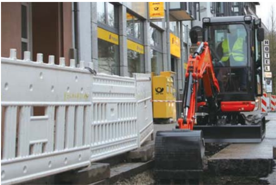
Mini excavators: used in civil engineering and other operations; especially useful in narrow work areas, such as city streets.
