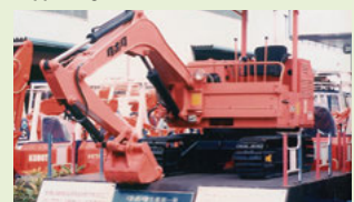
Fully revolving small hydraulic shovel, the base model for subsequent Kubota mini excavators
