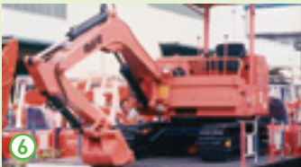
Fully revolving small hydraulic shovel, the base model for subsequent Kubota mini excavators
