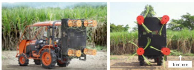
SLR110H mounted on a small tractor
