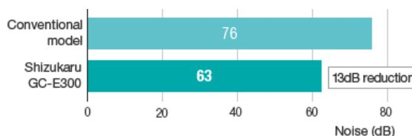
\* Noise values are compared at a distance 10m away from where the machine is operating
