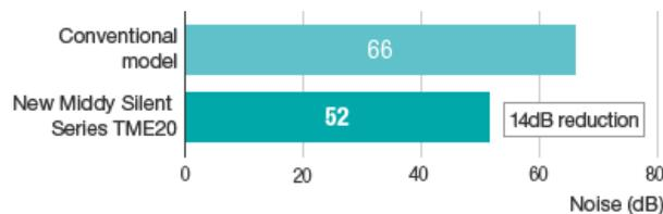
\* Noise values are compared at a distance of 7m away from where the machine is operating
