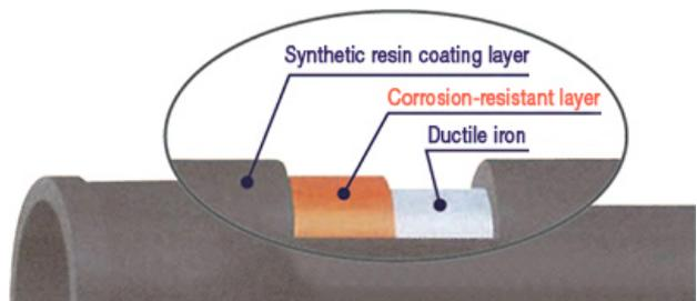
External corrosion-resistant coating C-Protect (conceptual image)
